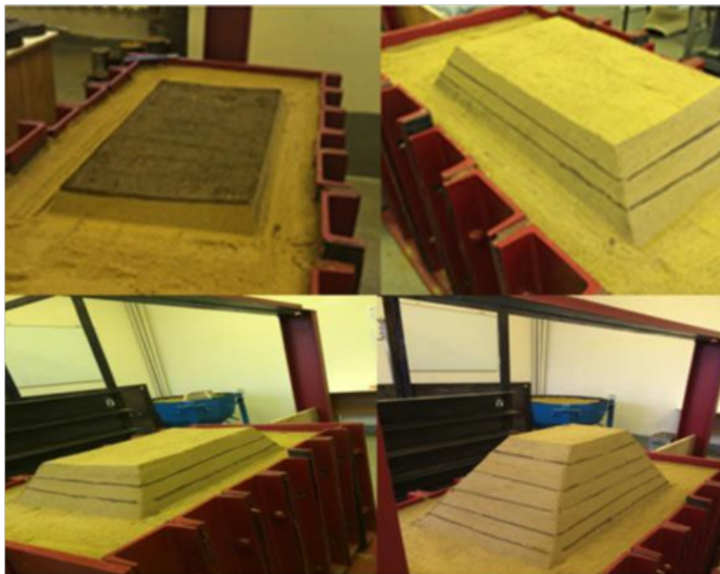
Figure 13. Dam model level-by-level placement without reinforcement
