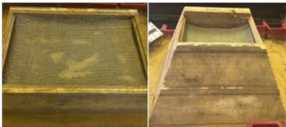
Figure 14. Reinforced dam model level-by-level placement
