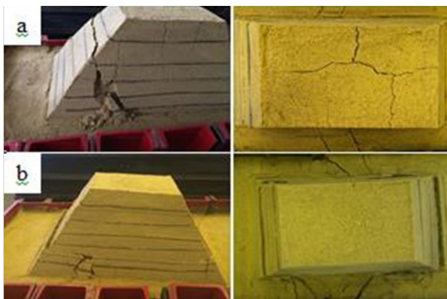
Figure 16. Comparison of stability modeling key stages for dam model (a) without reinforcement; (b) with reinforcement).
