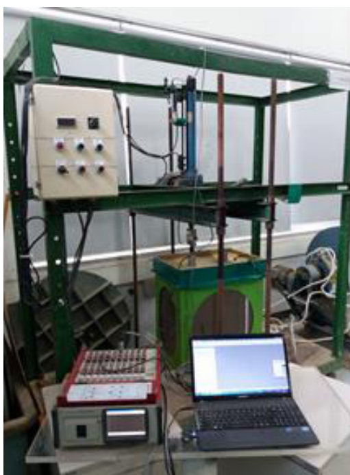
Figure 3. Static load tests for pile foundation in seasonally freezing soil
