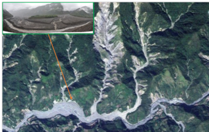
Figure 1 - Debris flows caused by Typhoon Morakot: Putunpunas River, SW Taiwan
