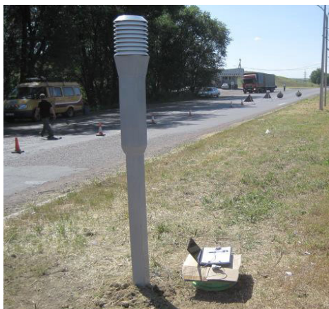
Figure 2 – Land part view of automatic measurement system of temperature and moisture on the highway «Almaty-Bishkek» (58 km + 895 m)
