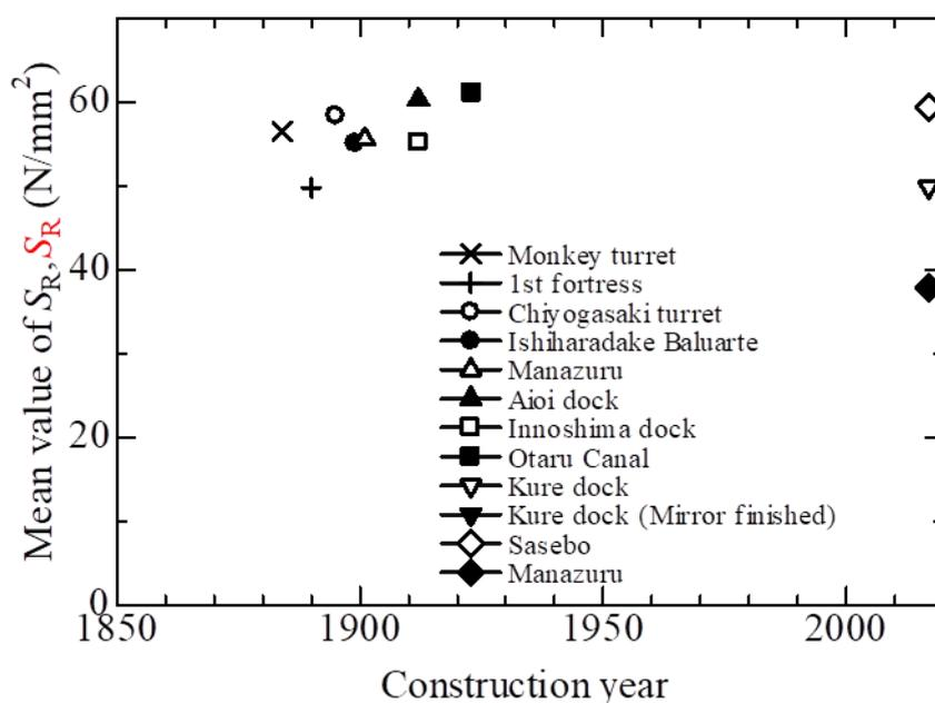
Figure 6. Relationship between SR and construction year(stones)
