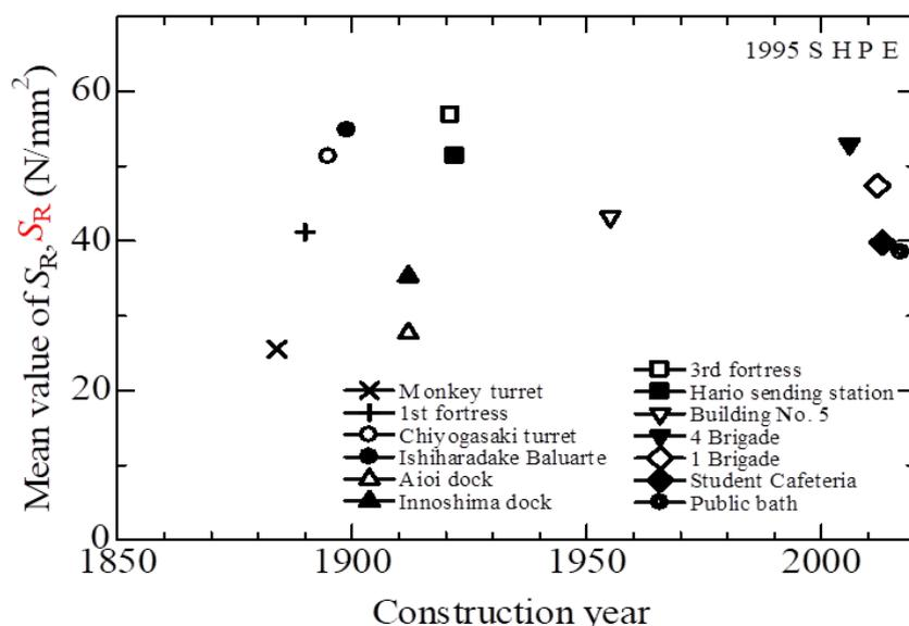
Figure 5. Relationship between  $S_R$  and construction year (concrete)
