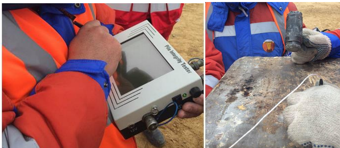
Figure3. PIT pile testing
