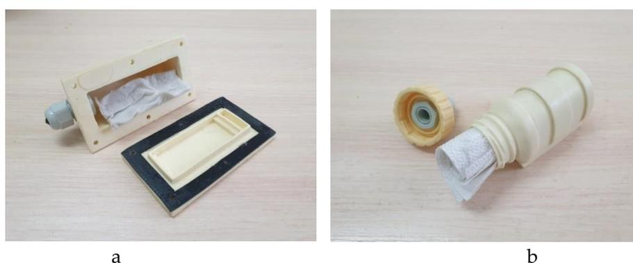
Figure 8. Water-resistance test results: a) wet tissue paper in the rectangular housing; b) dry tissue paper in the cylindrical housing
