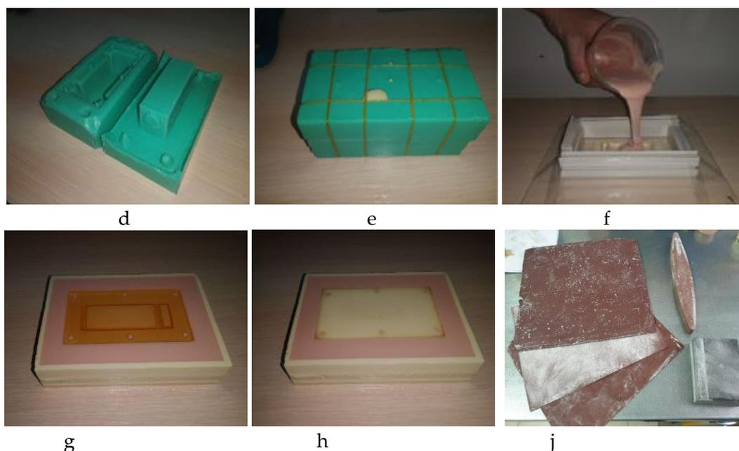
**Figure 1. Design and fabrication of a silicone mold for a rectangular housing: a) 3D design; b) prototypes; c) the pouring of silicon for upper part master-form; d) prepared silicone mold; e) cured upper part in the silicon master-form; f) the pouring of silicon for lower part master-form; g) the curing process of plastic in a silicone mold; h) cured lower part in the silicon master-form; j) polishing tools**
