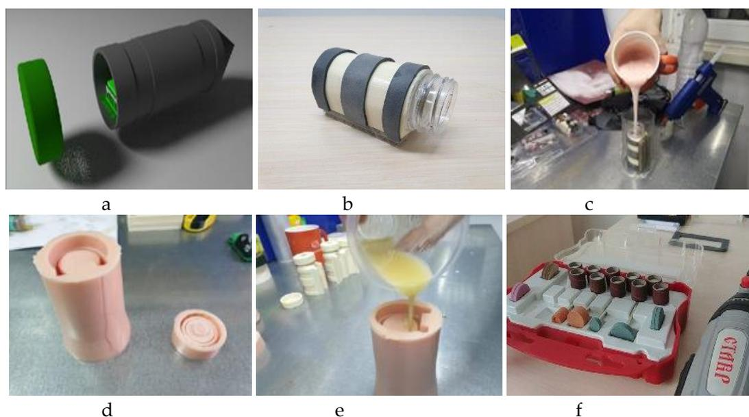
**Figure 2. Design and fabrication of a silicone mold for the cylindrical housing: a) 3D design; b) prototype; c) the pouring of silicon for master-form; d) prepared silicone master-form; e) pouring of plastic; f) polishing tools**
