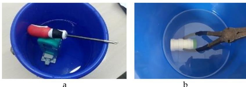
**Figure 3. Water resistance tests: a) rectangular housing; b) cylindrical housing**
