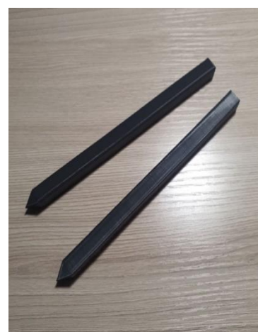
Figure 3. Process of filling the box Figure 4. Model piles made of plastic
