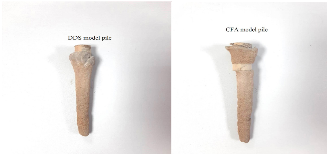
Figure 7: Model piles after static testing
