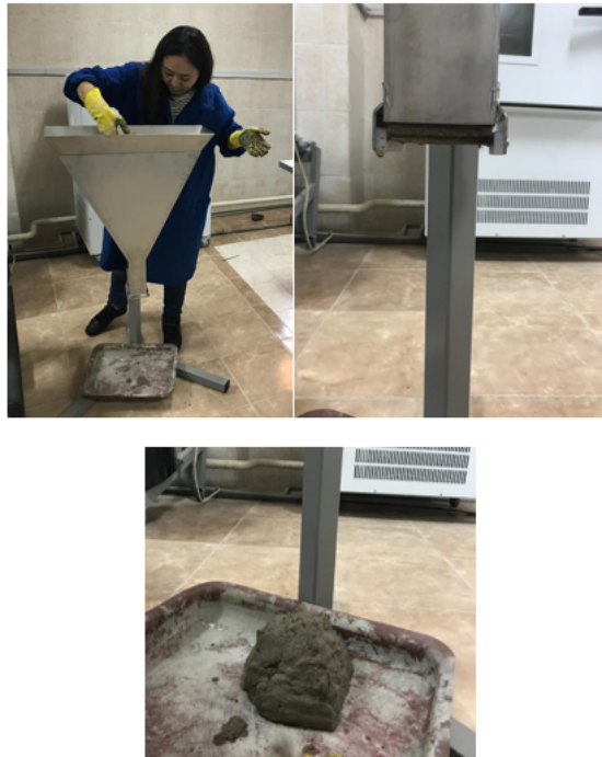
FIGURE 5 – Determination of the mobility of the sample
