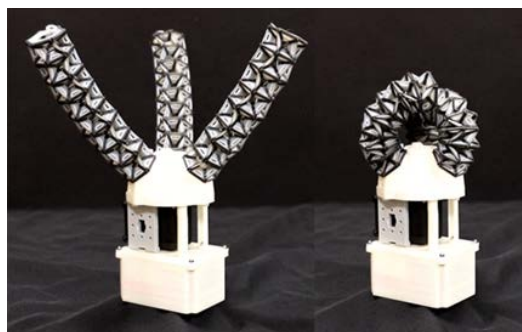
Figure 2. Underactuated cable-driven robotic gripper with three compliant fingers fully open (left) and closed (right) [11]
