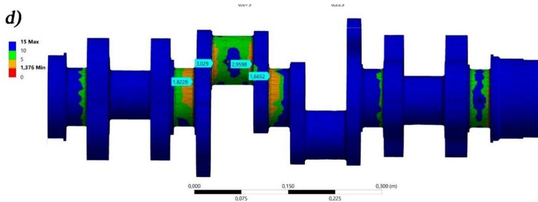
Figure 10. Fatigue strength safety factors
