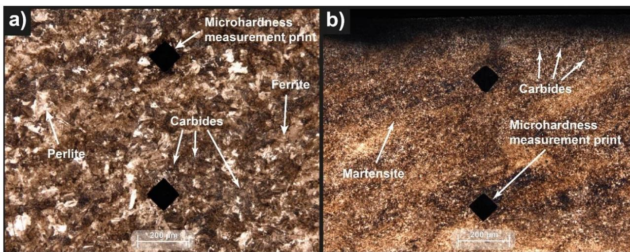
**Figure 4. Microstructure of 42CrMoVA Steel
