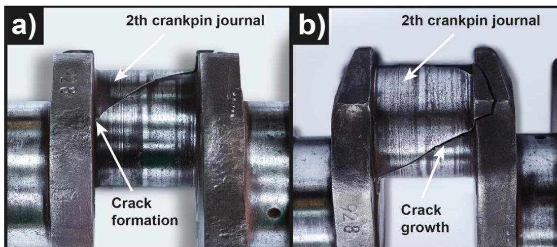
**Figure 3. Fatigue crack of the KamAZ-740 crankshaft
