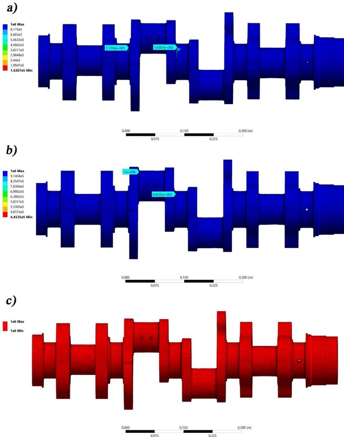
Figure 9. The number of available cycles of the KamAZ-740 crankshaft before fatigue failure
