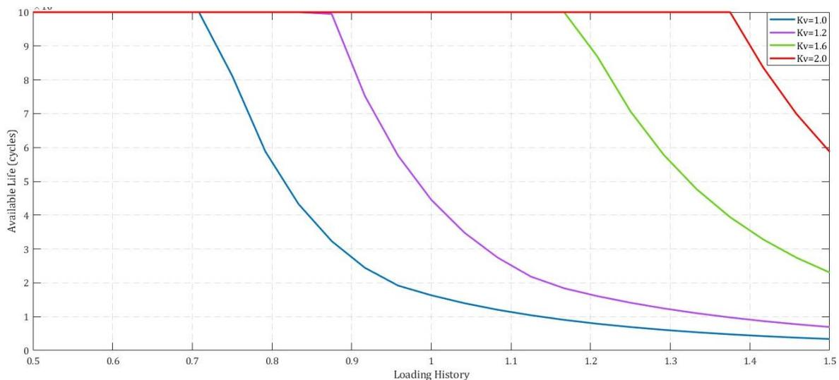
Figure 11. Fatigue sensitivity diagram
