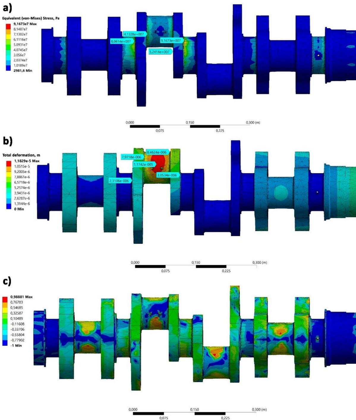
Figure 8. Stresses in the material of the KamAZ-740 crankshaft
