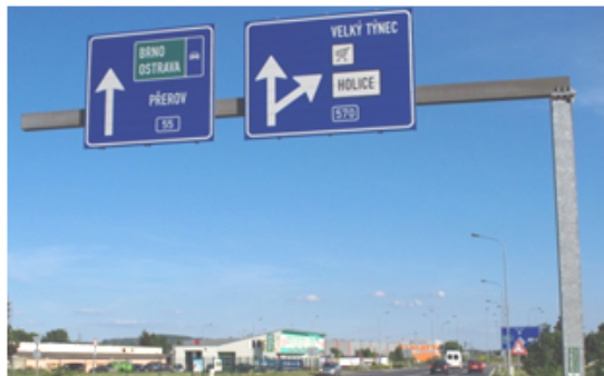
FIGURE 10 – Direction traffic sign for each traffic lane separately placed above entry lane on turbo-roundabout in Olomouc (roads I / 55 and II / 570, Czech Republic).
