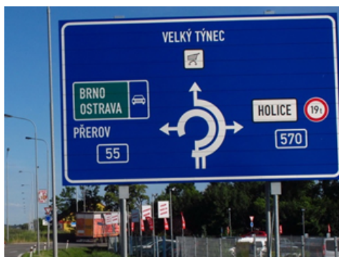
FIGURE 8 – One direction traffic sign showing all directions on turbo-roundabout in Olomouc (roads I / 55 and II / 570, Czech Republic).
