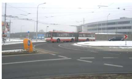
FIGURE 19 – Turbo-roundabout with over-runnable skirt (traversable aprons) in central island for use by buses and trolleybuses as well in Brno (Czech Republic).
