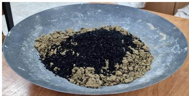
Figure 1. Engineering composite consisting of soil and shredded rubber (ground rubber)
