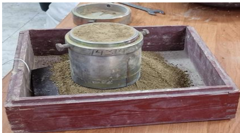
Figure 2. Sample compaction device made according to the typical design developed by the Research Institute “SOYUZDORNII”
