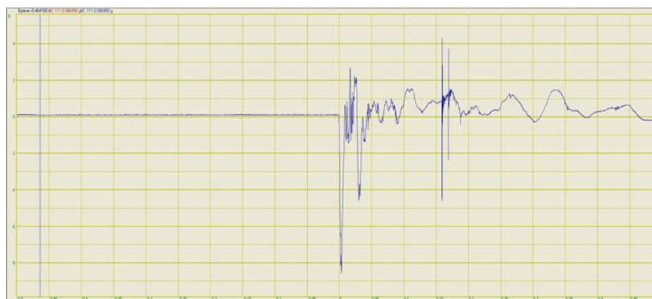
Figure 5. Acceleration diagram obtained during the testing of ground rubber
