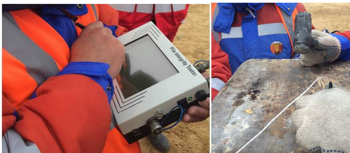
Figure3. PIT pile testing
