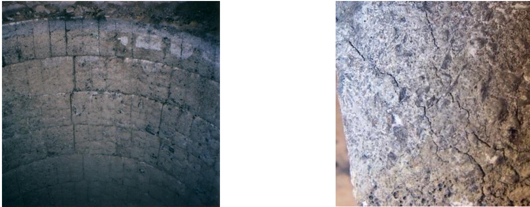
Figure 3. Cracks in the lining of a steel ladle
