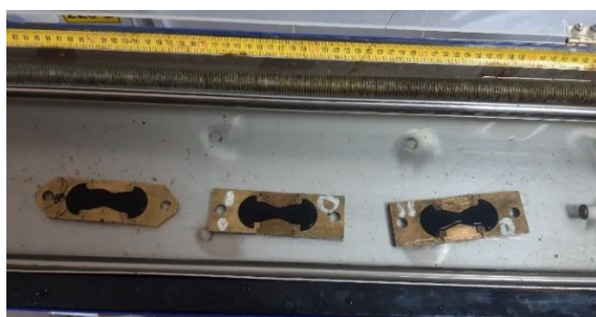
Figure 8. Photo of forms with samples of bitumen in the water ductilometer
