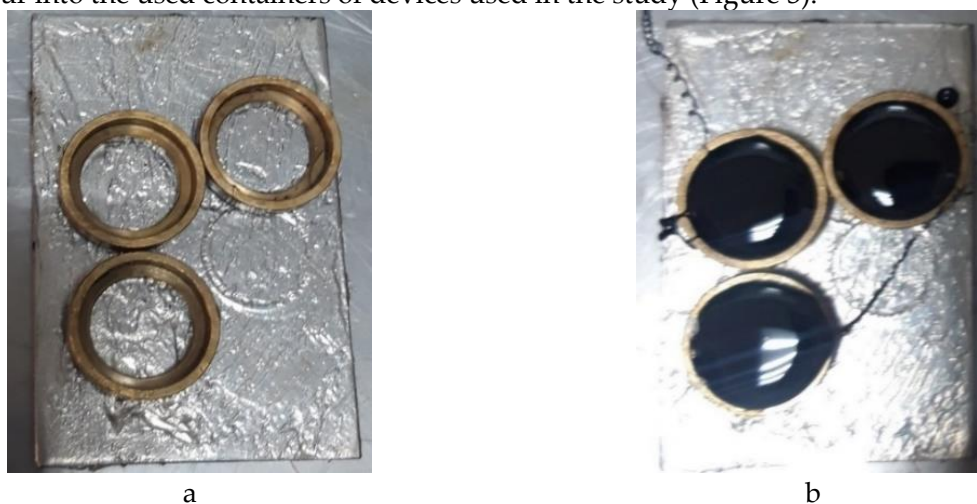
Figure 3. Forms for testing on the "Ring & Ball" device a) empty form; b) form with bitumen
