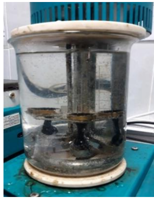
Figure 4. Bitumen testing process on the "Ring&Ball" device
