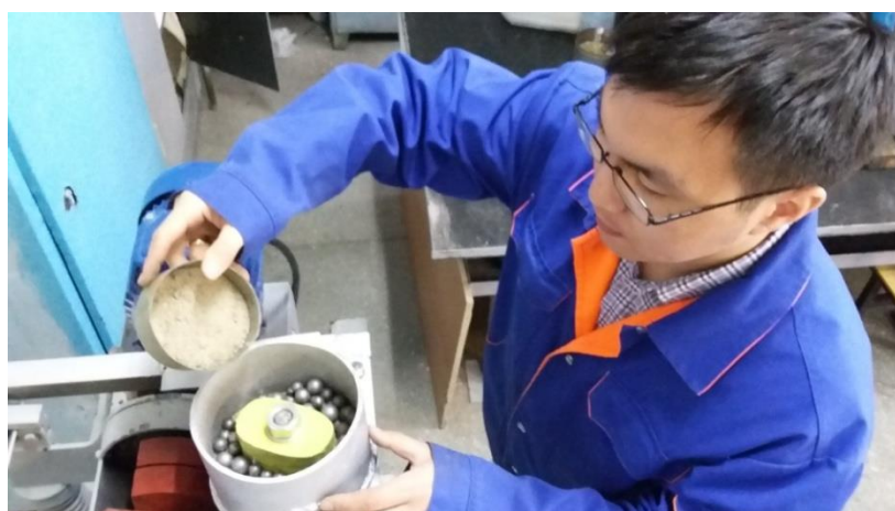
Figure 6. Filling the chamber with ground material
