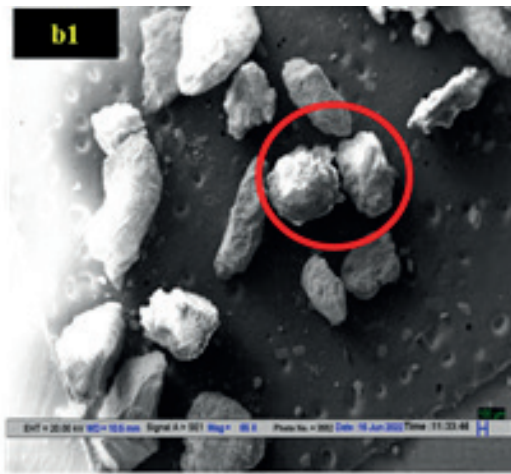
(b1) Double Coating (M: 65 \times , S: 0.6-0.425 mm)
