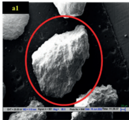
(a1) Double Coating (M: 65 \times , S:2.00 -1.00mm)
