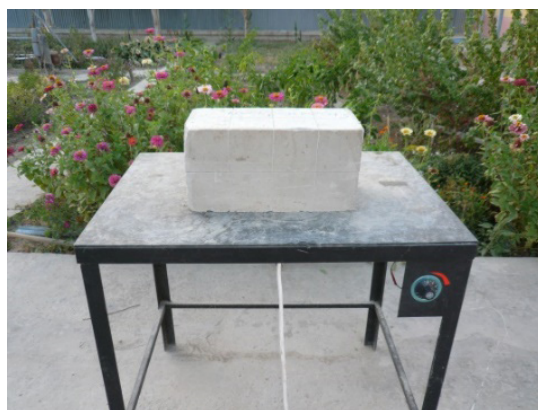
Fig.1 Apparatus for the laboratory with an electric mold heater and heliocoat
