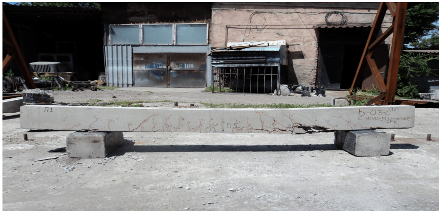
Figure 6. Beam failure with laminate reinforcement of the tensile zone
