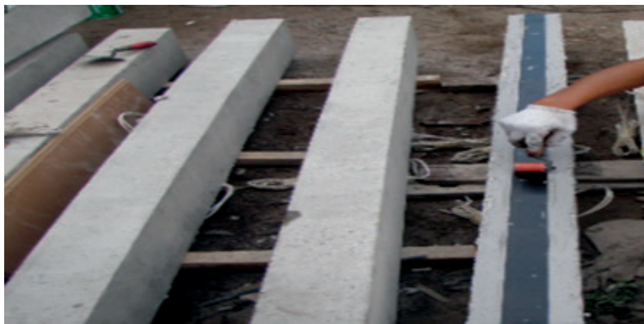
Fig.3 Process of strengthening
