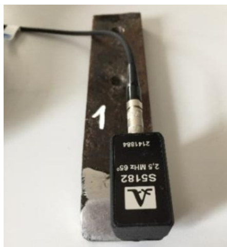
a) the process of measuring the working surface of the sample by the flaw detector sensor
