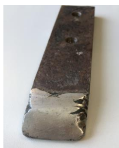
a) sample with hardened working surface by cladding with T590 electrode (front and back sides)
