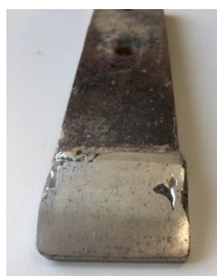
b) sample with hardened working surface by cladding with T590 electrode (full working part)
