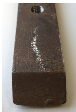
d) sample with thermally treated working surface according to factory technology
