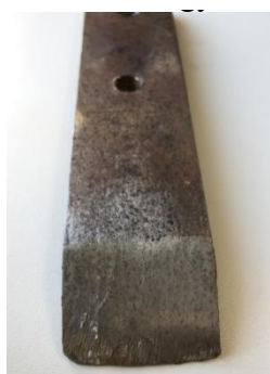
g) sample with thermally treated working surface according to factory technology
