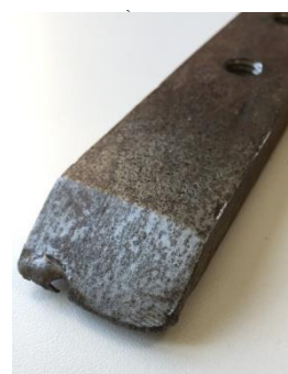
i) sample with thermally treated working surface according to factory technology
