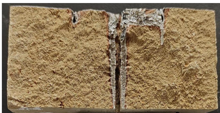
Figure 6 Fracture morphology of mudstone specimen
