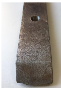
e) sample with thermally treated working surface according to factory technology
