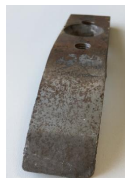
f) sample with hardened working surface by cladding with CS-1 electrode (sormite No.1)
