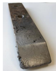
c) sample with hardened working surface by HFC hardening
