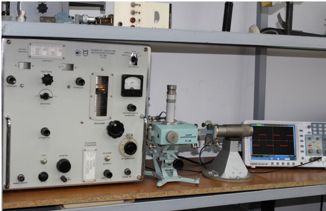
Figure 8. An experimental setup for studying dielectric characteristics of snow using a waveguide instrument line. In the left part of the figure, you can see the microwave generator connected to the P1-28 measuring line by the flange connection, then follows the waveguide section with snow and the short-circuited waveguide load with variable phase NKP-7; the oscilloscope is connected to the detector section of the measuring line
