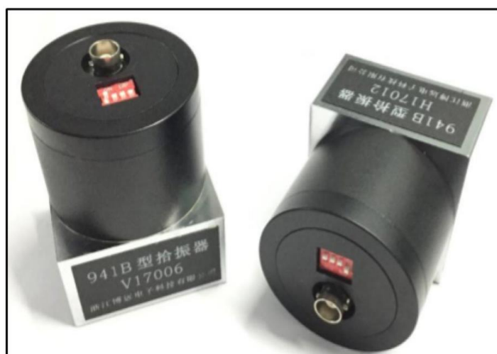
Figure 2 – Vibration sensor 941 B (manufactured in China) [8]
