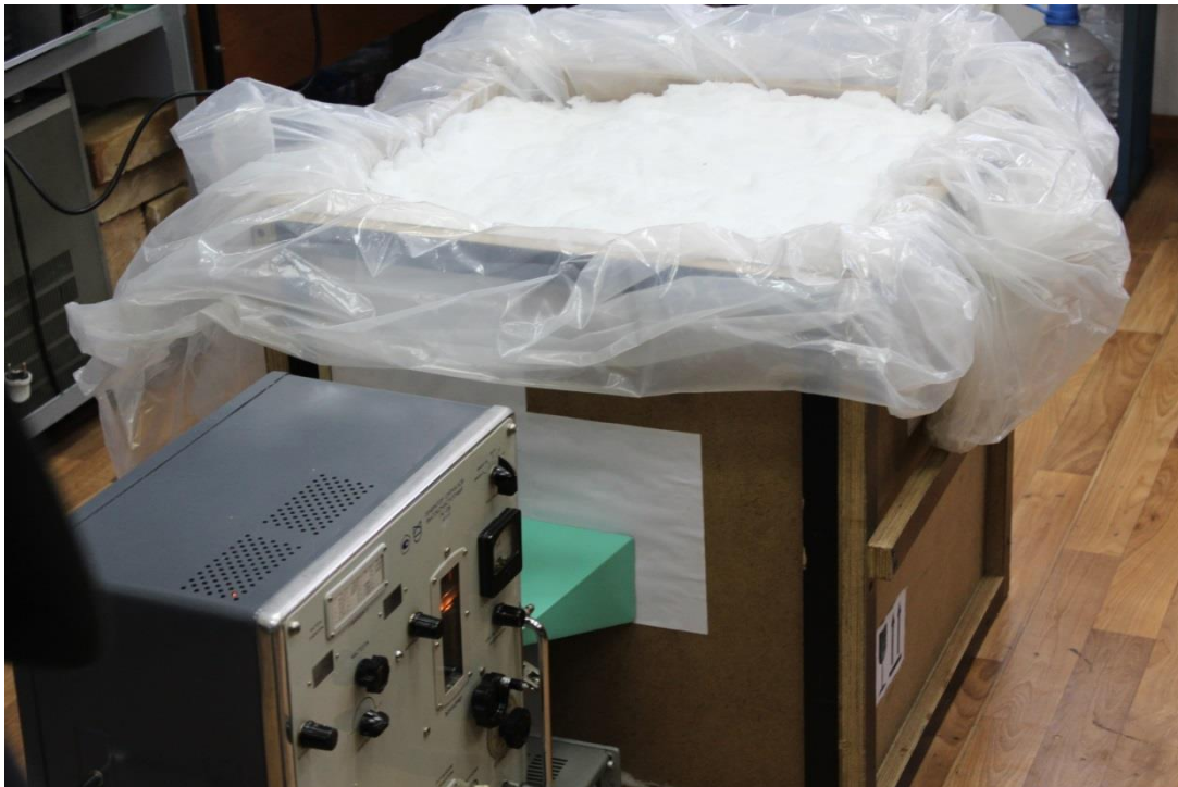
Figure 7. An experimental setup for measuring transmitted microwave radiation in case of the maximum filling of the container with snow (the snow layer thickness between the openings of horn antennas is 53 cm)
