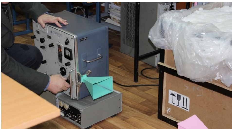
Figure 6. A photograph of the experimental setup for measuring microwave radiation without the container (the microwave generator connected to the transmitting horn antenna (light green color) and the receiving horn antenna (yellow))
