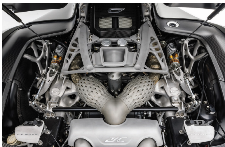
Figure 6. Printed part of the Czinger C21 motor [14]
