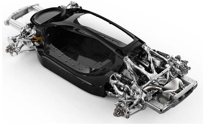
Figure 5. Printed Czinger C21 chassis [14]
