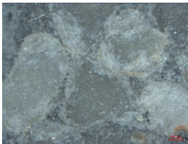
Figure 4. Microstructure of a fracture of a cement stone sample containing microsilica MKU-95
