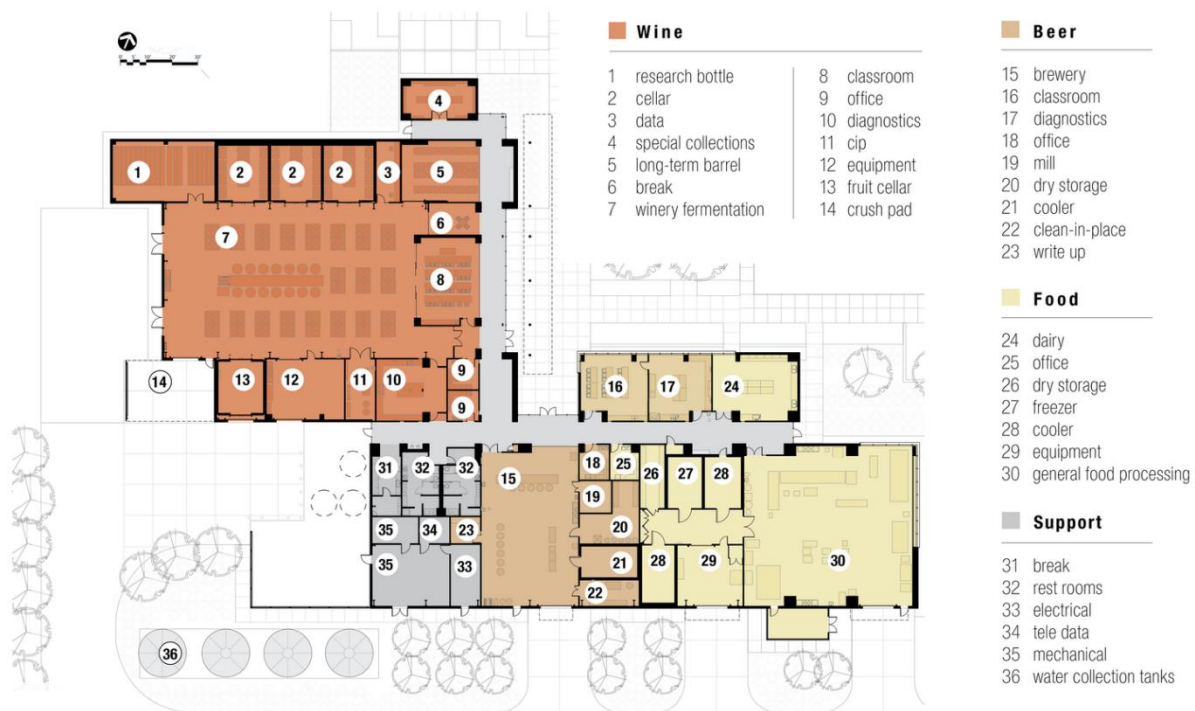
Figure 1. Functional zoning of the WBF Lab project
